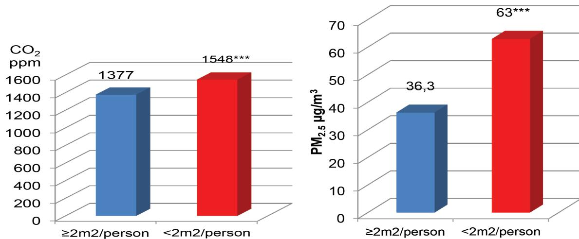
Figure 7. Mean  $\text{CO}_2$  concentrations measured in Hungarian classrooms with recommended ( $\geq 2 \text{ m}^2/\text{person}$ ) or reduced ( $< 2 \text{ m}^2/\text{person}$ ) floor space (SINPHONIE project)
